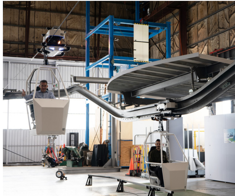
Project Swyft Small-Scale Proof-of-Concept Demonstrating Self-Propulsion Bogies, Cable-Rail Interfaces, Offline Stations. Source: Swyft Cities
