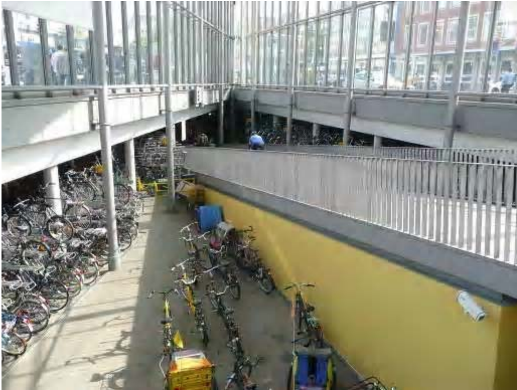
Interior view of bike parking facility at main train station in Muenster, with bike ramp from street level to parking level and direct access to train platforms
