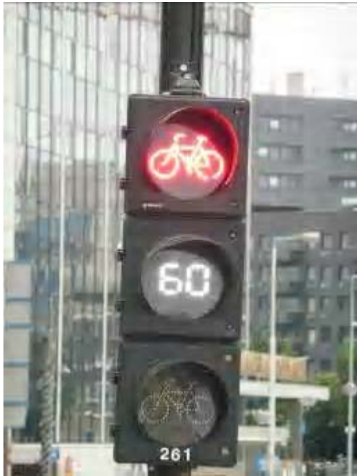
Bike traffic signal in Amsterdam that shows cyclists the number of seconds till they get a green light
