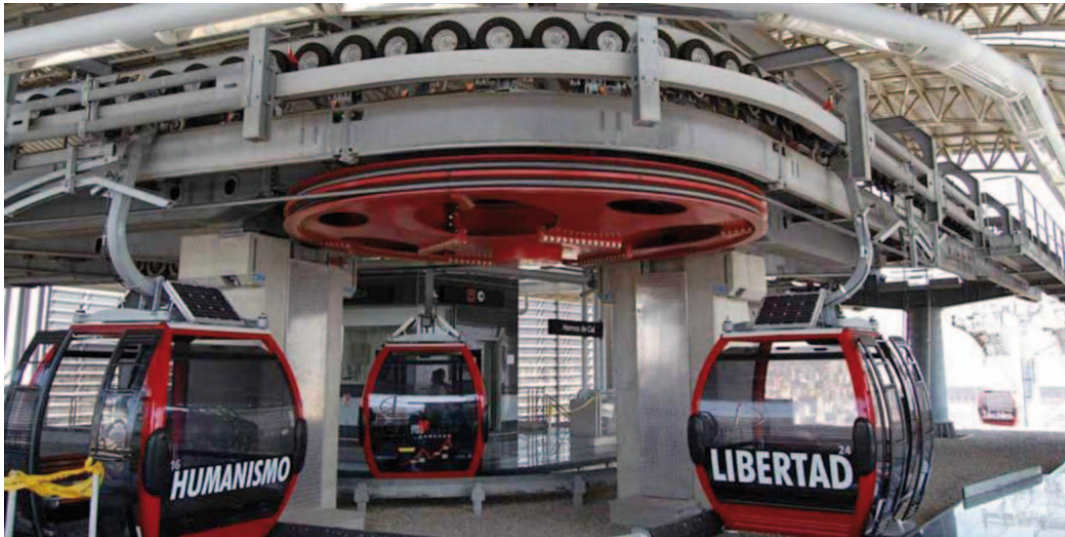
Plate 19: Passive deflection wheel at angle stations Source: CUP, 2016
