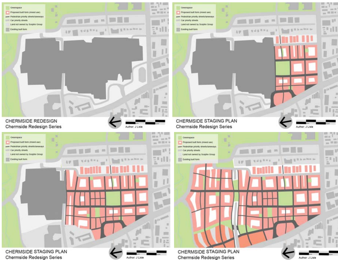
Figure 7: Staging of the redevelopment to allow continuation of most of the retailers during redevelopment from current form (top left) to Stage 1: Town Square and Entry Precinct (top right), Stage 2: Completion of Town Square and Main Streets (bottom left), Stage 3: Full completion (Figure 5) and Stage 4: Surrounding landowners embrace the concept (bottom right). (Jess Lisle 2016)
