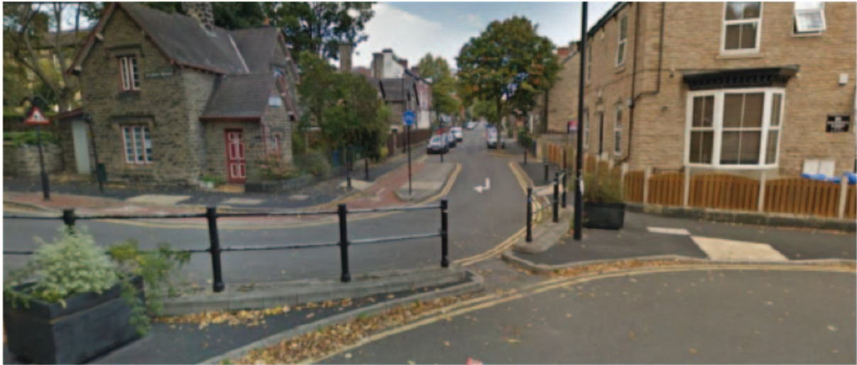
Figure 6: filtering of vehicular traffic to prevent straight-on traffic movements, Sheffield. © Google Maps
